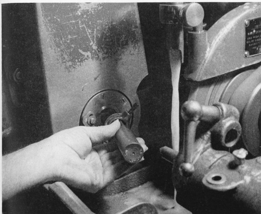
In the closeup above a Grinding Room operator demonstrates the proper way to insert a new piece of work into the grinding machine. Care at this time will eliminate most of the hazards from the grinding operation.
